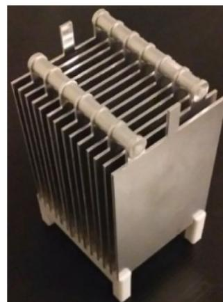
Fig. 2. Monopolar electrode configuration with a 5 mm inter-electrode distance, (anode: 7 electrodes, cathode: 7 electrodes). a) a schematic of electrode configuration, b) constructed electrodes.
