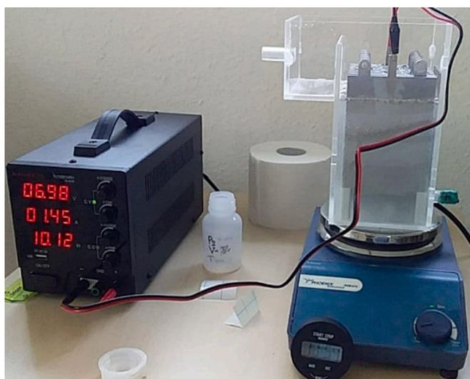
Fig. 3. Experimental setup for ECF process.
