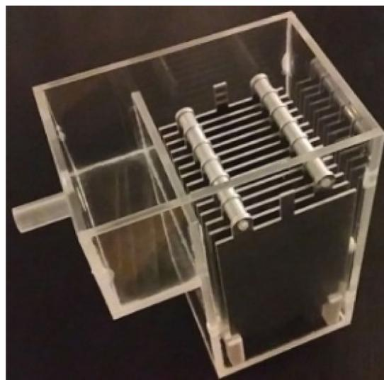
Fig. 1. A) a schematic of the cell and electrodes arrangement, b) constructed cell and electrodes.
