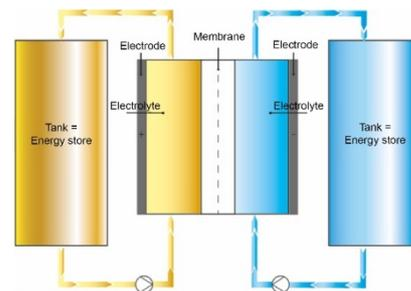
Fig.: Functionality of a redox flow battery
