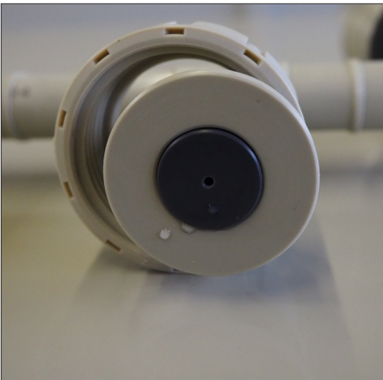
Figure 13: Inserted flow restrictor
