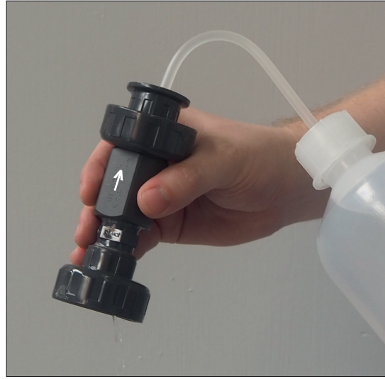
Figure 22: Flow limiter during flushing with deionised water
