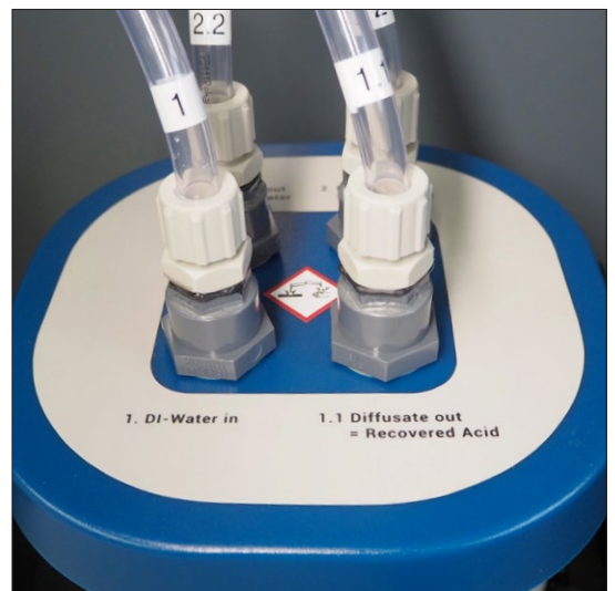
Figure 2: connected membrane modul
